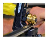
Accommodates a wider range of cable diameters without additional guide wheels.
