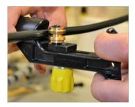
"T" handle design improves leverage & ergonomics during longitudinal or ring cuts.
